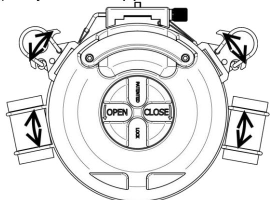
10) Tighten the support using the knobs
